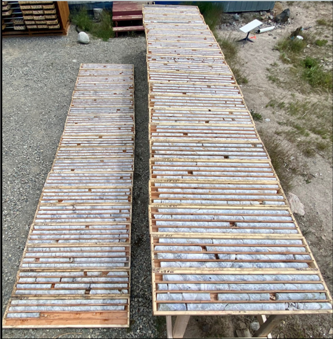
Figure 2. Spodumene-pegmatite between 202.5 and 381 m, Hole CS24-018, Cisco Property
