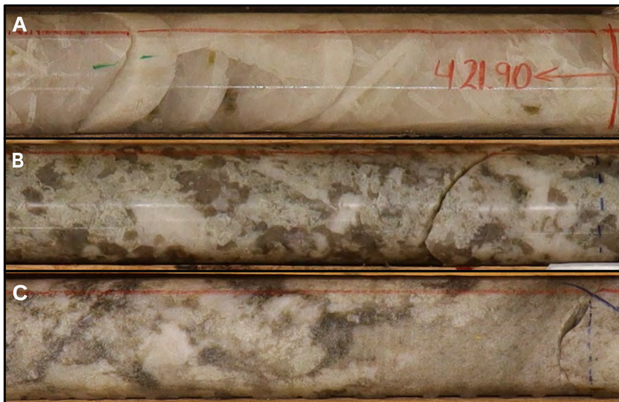
Figure 7-4: A) Coarse-grained, euhedral spodumene crystals in quartz matrix (~421.70-421.90 m in hole CS25-064). B) Spodumene-quartz intergrowths, interpreted to be magmatic in origin (~107.30-107.50 m in hole CS25-065). C) Fine-grained, “cloudy” or “spongy” spodumene-quartz intergrowths in a partially greisenized zone (~561.30-561.50 m in hole CS25-057)
