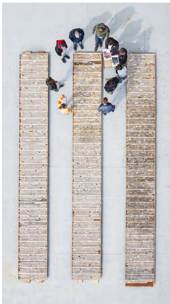
Figure 10-3: Drone photograph of CS25-044 drill core Shown is the 457.4 m core-length interval from 187.6 m to 645.0 m at 1.65% \text{Li}_2\text{O} . Core boxes are 4 ft long; personnel are shown for scale
