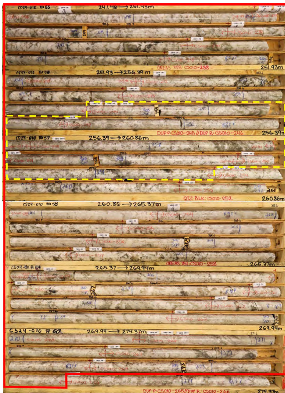
Figure 10-2: CS24-010: Spodumene pegmatite interval (25.1 m at 1.91% Li 2 O and 172 ppm Ta 2 O, red box) including 6.0 m at 2.54% Li 2 O and 162 ppm Ta 2 O (dashed yellow box)
