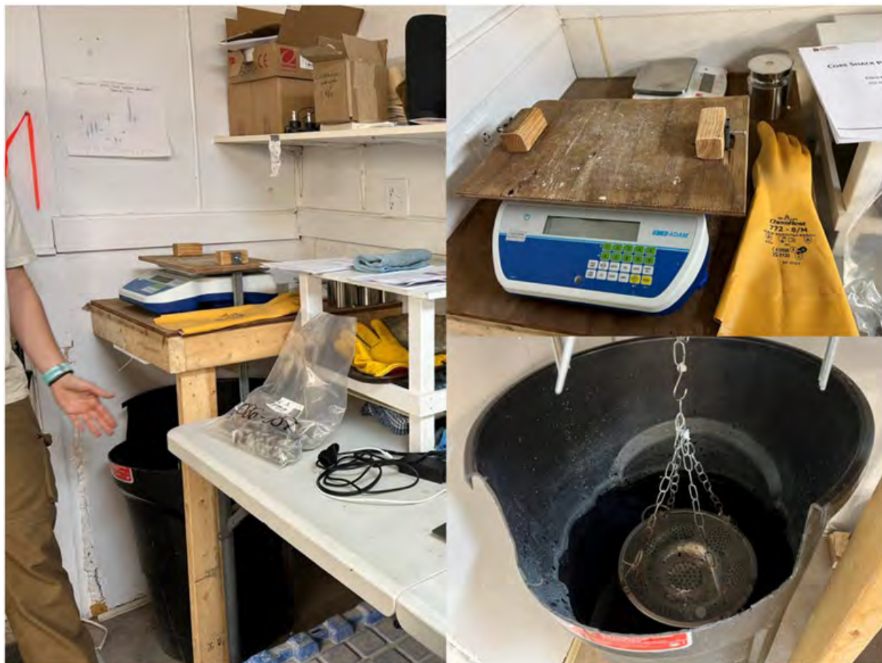
Figure 14-1: SG measurement set up employed by Q2 Metals
