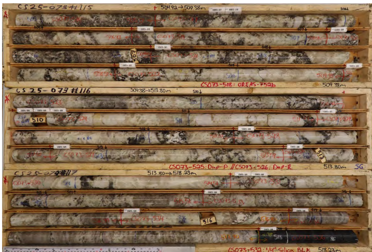
Figure 7-3: Drill core from hole CS25-073, showing commonly seen dm-scale textural and mineralogical variations
